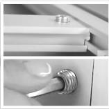
Now put the stabilizer in the frame while the lock is inserted in the inner slot of the profile. Then tighten the screws of the lock.
