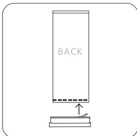
4. Pull back self-adhesive strip located on the media attached to the cassette. Slowly apply the strip to the back of your media ensuring its straight and secure.
