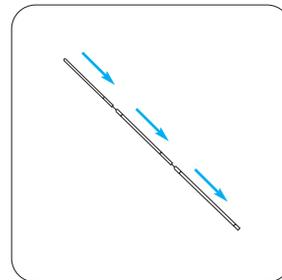
8. Remove the telescopic pole and fully extend. Push each section into the next to lock into place.
