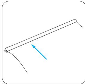
2. Slide media into the bottom end of the snap rail.
