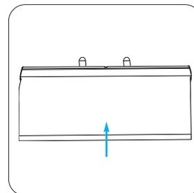
6. Slowly feed the media into the cassette keeping it as straight as possible whilst allowing the mechanism to wind.
