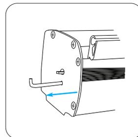
5. Hold the snap rail and the cassette securely and remove the pin from the side of the cassette to engage the mechanism.
