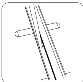
10. Ensure the pole is located onto the plastic lug securely. The lug sits inside the channel below the pole insert hole.
