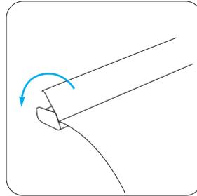
3. Push the snap rail closed ensuring the media is secure.
