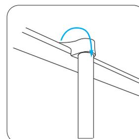
9. Locate the back channel of the snap rail onto the plastic adaptor at the top of the pole. Repeat steps in reverse to disassemble.
